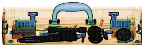
*Presented side by side, high-quality top and side views of a screened bag enable operators to discern threats confidently. The system automatically places a red box around possible explosives to alert operators immediately.*
